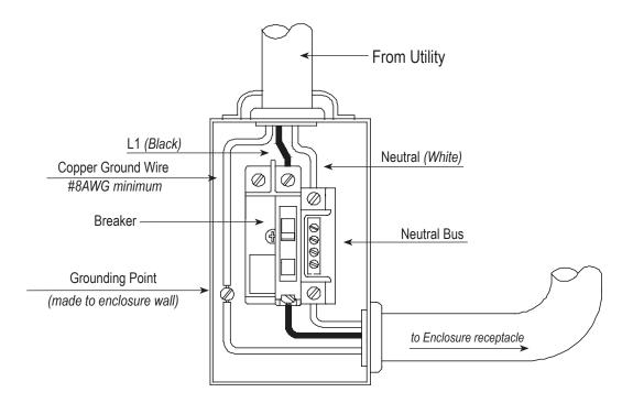
Fig. 2-6, 120Vac Service Entrance Wiring
