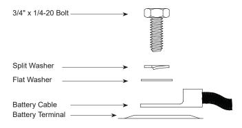
Fig. 2-10, Hardware stack-up, Threaded Battery Insert
