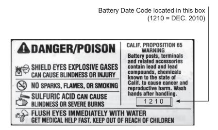
Fig. 2-9, Battery Identification Label
