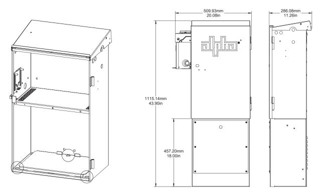
Fig. 2-5, Enclosure-to-Pedestal Mounting
