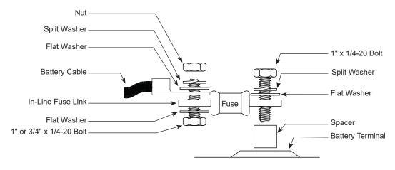
Fig. 2-11, Hardware stack-up, Threaded Battery Insert with optional in-line fuse
