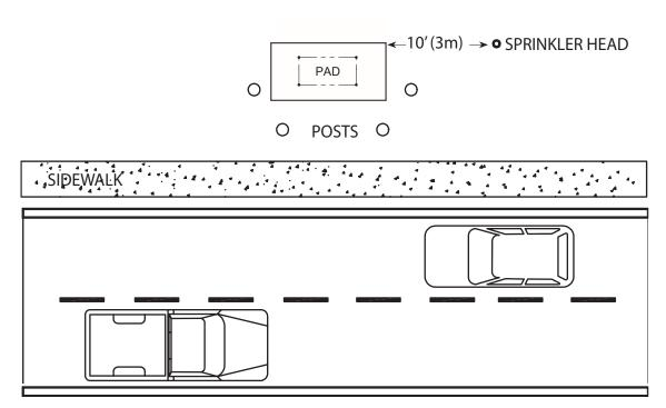
Fig. 2-2, Ground-mount Positioning and Safety
