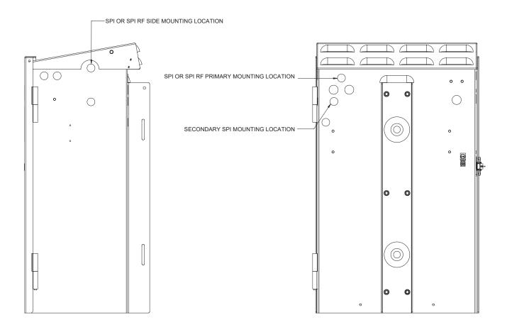
Fig. 2-8, SPI and SPI-RF Mounting Locations
