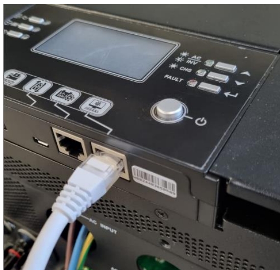
Figure 1: Left: Connect the white cable to the inverter at the RS232 port; Right: Connect the end of the cable labeled 'FernLite' to the FernLite
