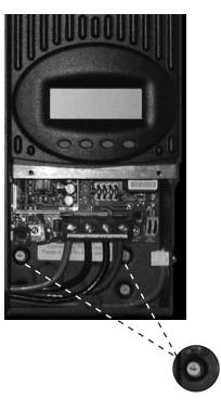
The MX Charge Controller attaches to the chassis using three #10 X 3/8" sheet metal screws included in the hardware kit. Two are inserted from inside the MX and the third through the hanger on the top of the MX.
