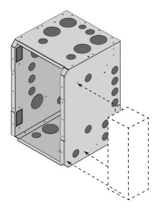
With the Mounting Plate and the hanging screws (for the FX Inverter/Chargers) inserted, install the FXs.
