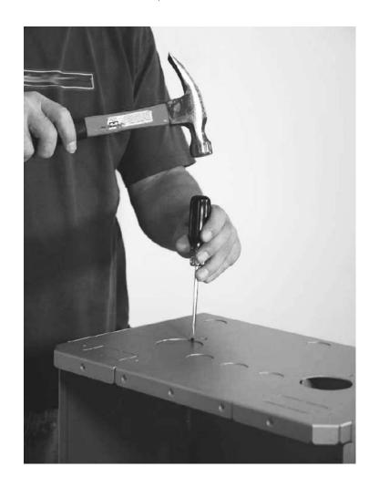
Note: It is easier to remove the appropriate side knockouts from both the AC and DC chassis before installing either of them. If needed, the back knockouts must be removed before installation.
