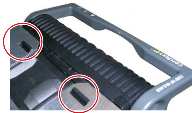
Figure 20 — Locking the Front Panel in Place
