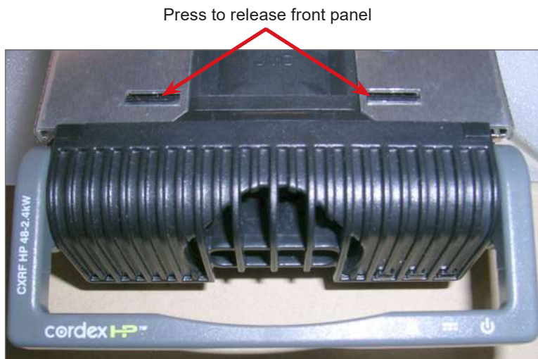
Figure 17 — Removing Front Panel from Rectifier
