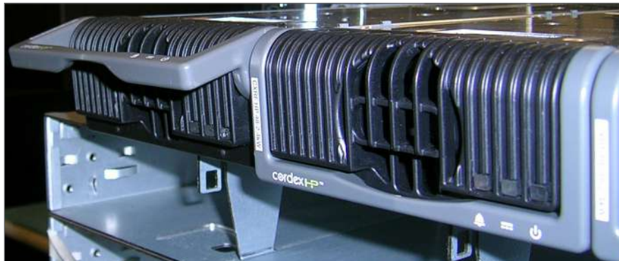
Figure 4 — Locking Handle Disengaged/Engaged
