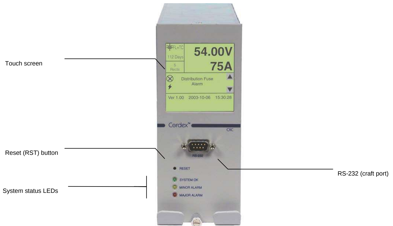
Figure 4–Cordex CXCM model system controller front panel
