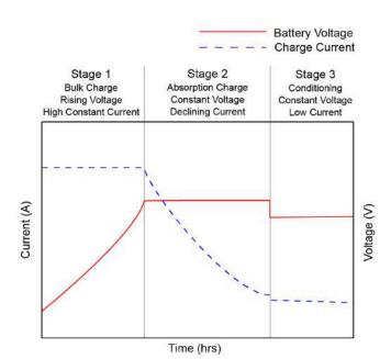
Figure 50. Three-Stage Charging Cycle
