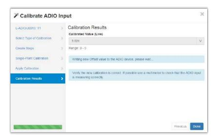
Verify that the new Calibrated Value matches the digital voltmeter reading. Click Done to close the Wizard.
