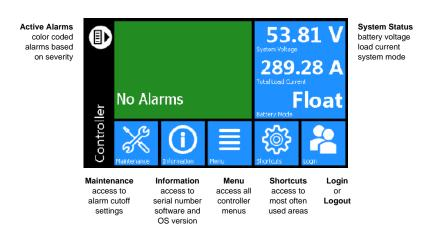
The upper-left area of the dashboard is the **Alarm** tile. If there are active alarms the LCD will show the top three active alarms.
