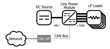
Figure 64. Example eLImiter+ System
