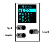
Figure 42. In-Shelf Controller Buttons: Horizontal Mount
