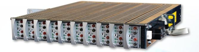
The CSM46 is a +/-190V to 48V DC-DC converter system designed for remote sites in network or line powering architectures. The compact modular design makes the CSM46 ideal for remote applications such as xDSL and FTTx.
