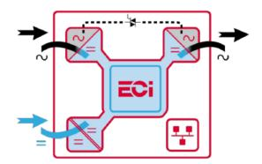
The ECI technology eliminates all single points of failure with full scalability; up to 32 modules in parallel and high efficiency of up to 96% in AC to AC conversion, and above 94.5% in DC/AC conversion, hence reducing operating costs.
