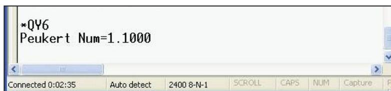
To change the Peukert Number to 1.1345 for example, type " \*ST6:1.1345" at the command line and press "Enter".
