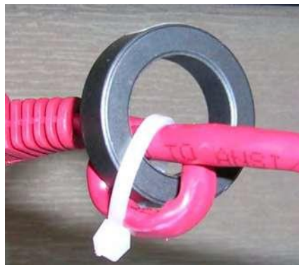
Figure 19 — Ferrite ring installed on RJ45 network cable
