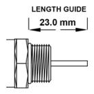
Screw the male cable connector (external fitting) into the 5/8" female connection. The center pin is automatically seized by the female connector. Prepare and attach the coaxial hardline feeding the HFC plant to the male cable connector as per the manufacturer's instructions.
