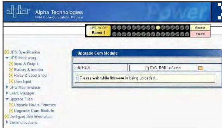
Figure 45 — Alpha UPS Monitor: Upgrade Communication Module
