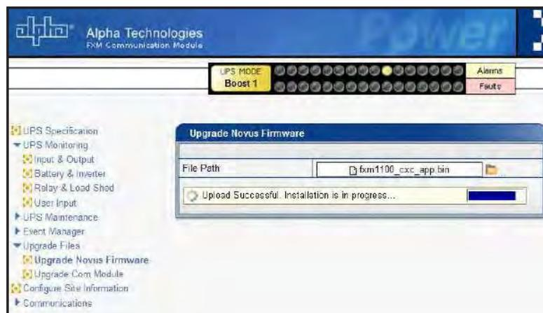
Figure 44 — Alpha UPS Monitor: Upgrade Firmware
