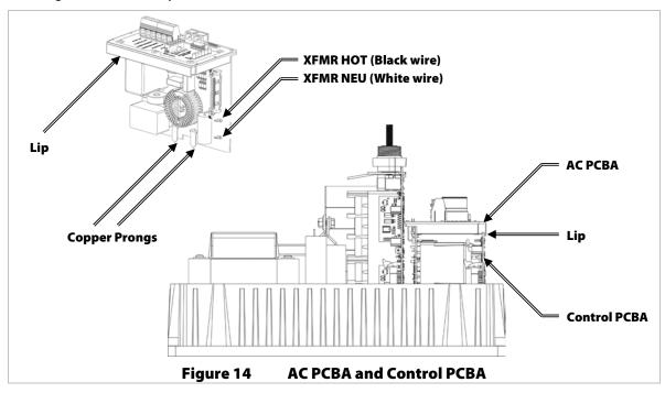
6. With the AC PCBA lifted as high as possible, guide the Control PCBA into its slot in the chassis. Lower the AC PCBA over the top of the Control PCBA. As shown in Figure 14, there is a "lip" on the AC PCBA that fits over the top of the Control PCBA.
