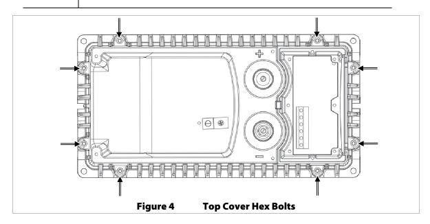
8. Carefully lift the inverter cover, just far enough to locate the fan wire.
