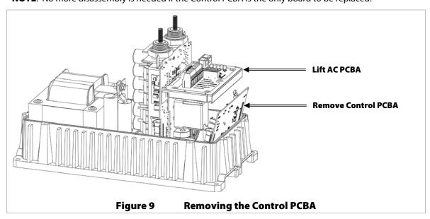
14. Before removing the AC PCBA, using a pair of long-nose pliers, disconnect the white and black AC output wires connected at the bottom of the board. (See Figure 10 for the location of the wire connectors.) Remove the AC PCBA.
